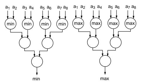
c. The following picture is showing the dependency graph for the minimum and maximum search by using of minmax–nodes. These minmax–nodes can simultaneously determine the minimum and maximum of two input operands. The
