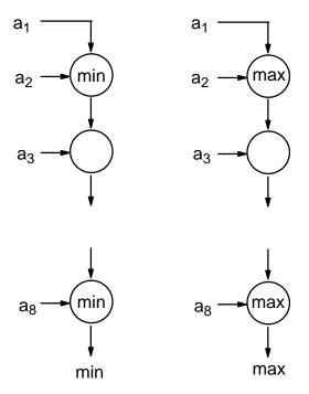
b. The hierarchical structure of the maximum and minimum search for 8 input operands with separated trees is shown in the following picture. The effort with 7 nodes for minimum and maximum search is the same like the sequential approach in a.) whereas the delay is reduced from 7 steps to 3 steps.
