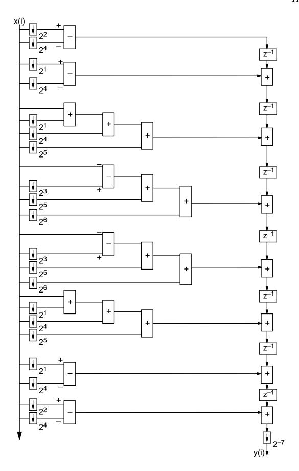
b. The following picture shows the complete FIR filter after factorization (see Figure 10.1.3) and utilization of the symmetric impulse response (see Figure 6.2.13). The number of adders/subtractors needed for the complete FIR filter can be reduced from 23 to 11.
