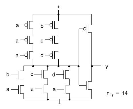
By factoring out of the variable a you can save transistors in the pull-up as well as in the pull-down path.
