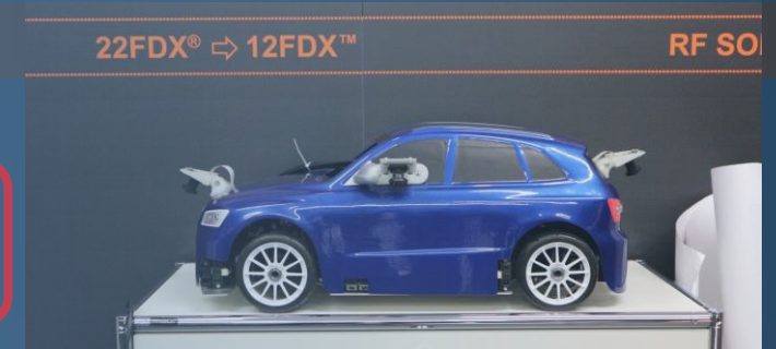
360° Surround View Demo Setup Demo-Car with 4 cameras
